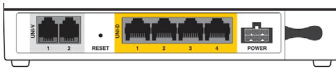
Plug the other end of this Ethernet cable into the WAN port on your modem/router. This may also be labelled as INTERNET or WAN/LAN. The Ethernet cable is larger than a telephone cable. DO NOT use the telephone cable to plug in your modem/router to the nbn™ FTTP Network Termination Device (NTD).
